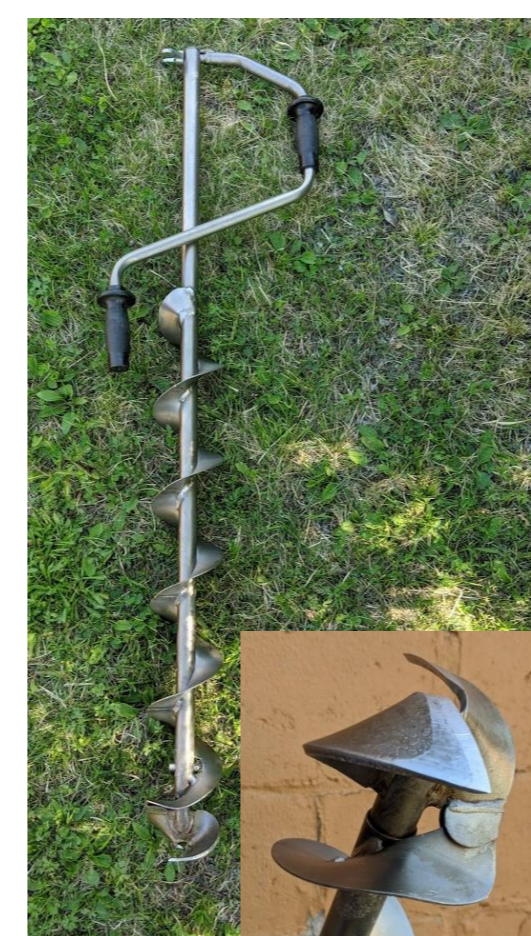
Fig.4 Titanium ice drill
