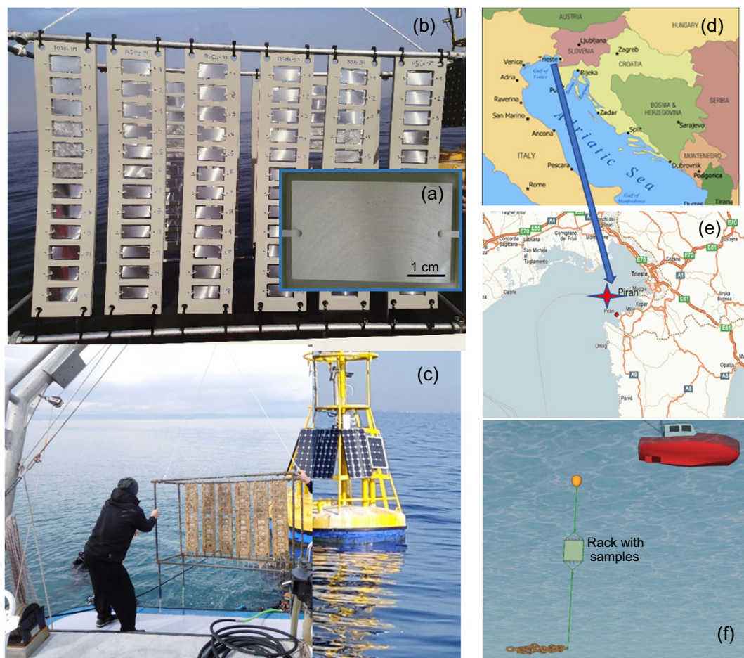
FIGURE 2. (a) Individual sample, (b) frame with racks with samples, (c) removal of the racks with samples from the seawater near the buoy, (d, e) maps of the immersion site (coordinates 45^{\circ} 32.925' N, 13^{\circ} 33.042' E), and (f) positioning of the racks with samples at a depth of 20 m.
