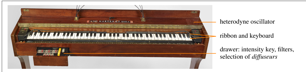
Figure 1: Ondes 169 (E.991.8.4) from 1937 and its principal components [Photo © Claude Germain, Philharmonie de Paris]
