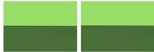
Figure 15: Zoom-in of the top edge of the KCS hull model. Left: smoothed edge with consequent oscillations due to the G^1 continuity. Right: sharp edge achieved by imposing C^0 regularity along the sharp edge.
