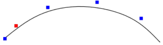
Figure 2: Schematic of a cubic B-spline with knot vector [0,0,0,0,1,2,3,4,\dots] . The slope control point is shown in red, and all other control points in blue. The location of the red point influences the shape of the spline only within the first two knot spans.
