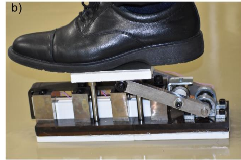
Figure 6 : Testing of the device with a true step. a) Experimental voltage (dashed line) and current (solid line) as a function of time. b) Photograph of the device when stepping on it.
