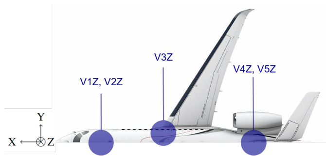
Fig. 1 Position of the 5 accelerometer channels considered in this study.
