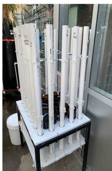
Figure 1 left: Biofilter column design; right: Real constructed biofilter columns in glasshouse
