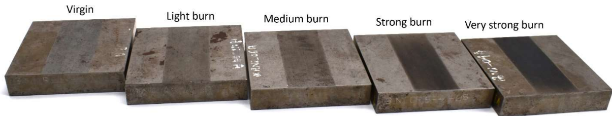
Fig. 2 – Illustration for the five grinding burn levels.
