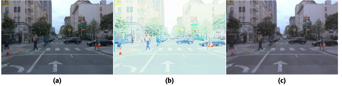
FIGURE 8. From left column to right column: the input normal-light image, the extracted raw illumination and the reflectance. Textural details such as the frontage of the buildings end up in the reflectance which demonstrates the quality of the decomposition model.
