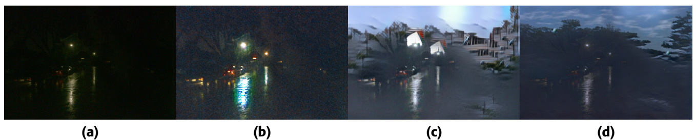
FIGURE 7. Style transfer and data augmentation methods with from left to right: Fig. 7a The input image, Fig. 7b CoMoGAN [39], Fig. 7c ManiFest [40], Fig. 7d MUNIT [22] trained on the Waymo dataset. These style transfer methods do not preserve the integrity of the scene in the input image and add hallucinations.
