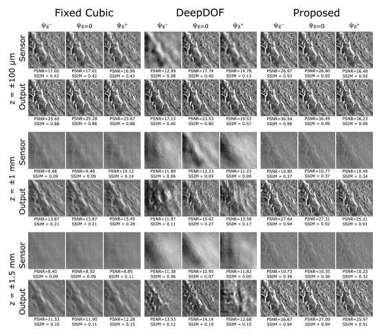
Fig. 4: Simulated performance of a cubic-mask-enabled computational 4f system, DeepDOF model, computational EDOF microscope, optimized for various target depths. For all DOFs, our method shows superior performance.
