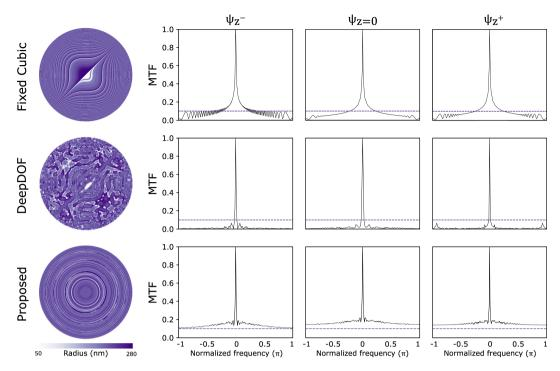
Fig. 5: The optimized metalens radius maps, as well as the MTFs at three distinct depths, are presented for the existing and proposed methods, encompassing the maximum defocus values within the 3 mm DOF scene and the in-focus depth.
