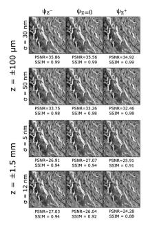
Fig. 6: Reconstruction results for increasing radius and height-map fabrication error levels.
