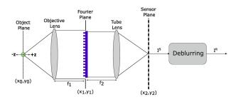
Fig. 1: A 4f system computational EDOF microscope model that combines the optical module, sensor, and D-CNN.
