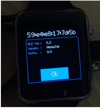
Fig. 5. Lilygo T-Watch running our custom firmware.
