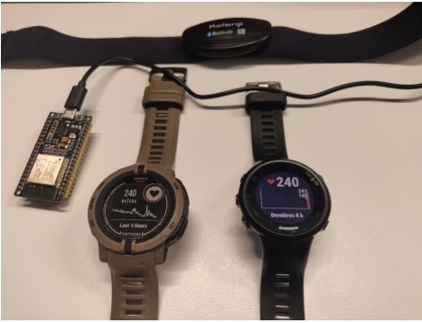
Fig. 7. Experimental setup for malicious ANT+ packet injection.
