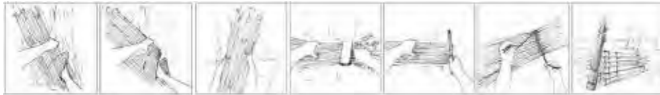
Operating chain 1: From reed to bale. © LMdP 2022.
