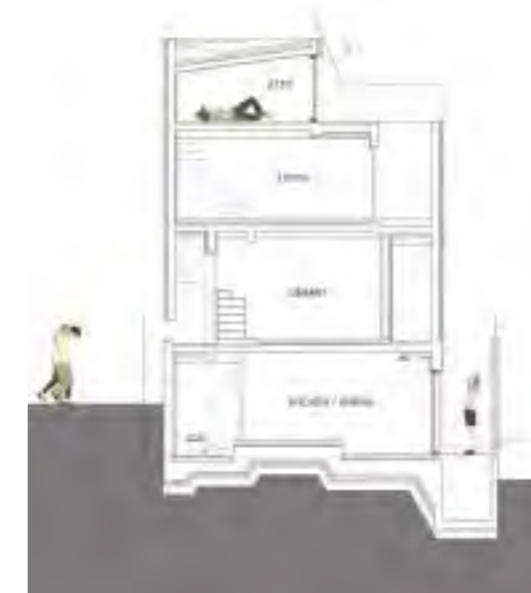
Image 3.03 The Section of the House. Source: Tiny Second Home in Urban / mundoehoje | ArchDaily
