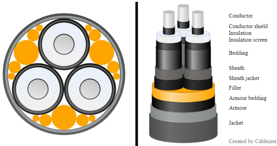
Figure 2 Cross-section and 3D view of a cable similar to the one used in our paper. Reproduced with the permission of Cableizer
