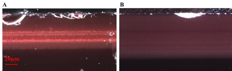
**Fig. 1 – Dark field reflection optical microscope image of (A) TDM; (B) CB6 showing the presence of metallic copper nanoparticles.**
