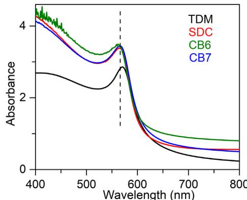
**Fig. 3 – UV-Vis absorption spectra taken in transmission mode showing the SPR extinction band at 560 nm characteristic of metallic copper nanoparticles (20–50 nm). The spectrum corresponding to TDM appears slightly red shifted due to the large particle size (50–150 nm).**
