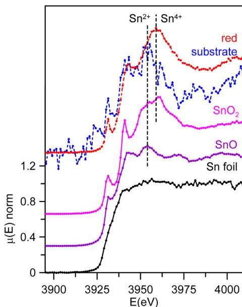
**Fig. 6 – Sn L<sub>3</sub>-edge spectra of SDC colourless substrate glass and red glass layer and Sn standards. Sn<sup>4+</sup> predominates in the red glass layer while Sn<sup>2+</sup> predominates in the colourless substrate glass.**
