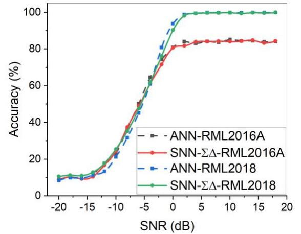
Fig. 7 Classification accuracy at different signal-to-noise ratios (SNRs) for the ANN (dashed) and SNN- $\Sigma\Delta$  (solid). For the SNN- $\Sigma\Delta$ , the order is set to two on the RADIOML (RML) 2016A dataset and three on RADIOML 2018 dataset. The OSR is 32.
