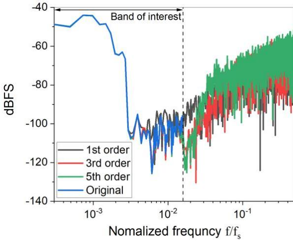
Fig. 6 Frequency response of the modulated outputs by the  $\Sigma\Delta$  modulator of different orders. The modulation class of the original sample is QPSK and the SNR is 18. Only the in-phase component of the sample is presented.
