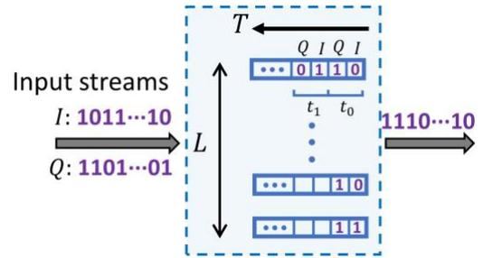
Fig. 10 Input buffer design for  $\Sigma\Delta$  modulated input streams. Each buffer saves one group of interleaved consecutive input streams from the two channels. All the data at the same time stamp (e.g.,  $t_0$ ) are then streamed out to the first layer through a FIFO channel.
