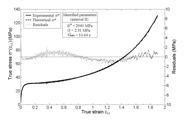
Figure 7: Experimental data, fitted curve (Eq. 15) and residuals obtained when identifying parameters  $E^u$ , G and  $\tau_{\max}^T$  on interval II (Specimen  $A_{//}$  - Strain rate of  $2.5 \times 10^{-3} \, \text{s}^{-1}$ ).
