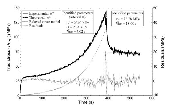
Figure 9: Tensile test followed by a relaxation for specimen B. Experimental data, fitted curve (Eq. 15) and residuals plotted as a function of time. Identified parameters are  $E^u$ , G,  ${\tau_{\max}}^T$ ,  $\sigma_{\infty}$  and  ${\tau_{\max}}^R$  - Strain rate of  $5\times 10^{-3}\,\mathrm{s}^{-1}$  (400 s correspond to a true strain of 2).
