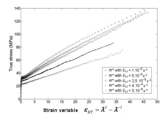
Figure 4: True stress  $\sigma^*$  versus strain variable  $arepsilon_{HT}$  (specimen  $A_{//}$  - Different strain rates).
