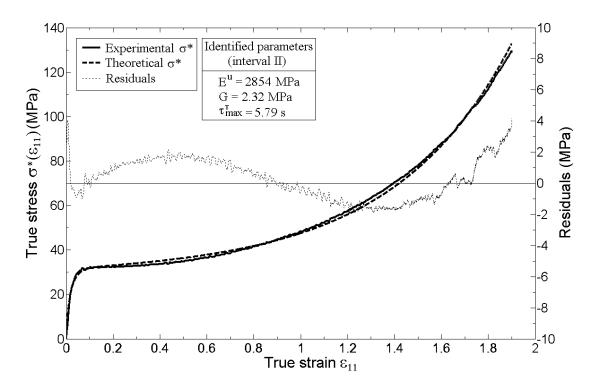
Figure 8: Experimental data, fitted curve (Eq. 15) and residuals obtained when identifying parameters  $E^u$ , G and  $\tau_{\max}^T$  on interval II (Specimen  $A_{//}$  - Strain rate of  $5 \times 10^{-3} \, \text{s}^{-1}$ ).
