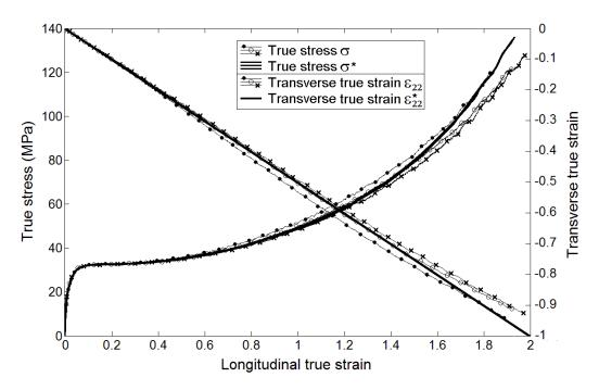
Figure 2: True stress  $\sigma$  or  $\sigma^*$  (left axis - the latter in solid black) and transversal true strain  $\mathcal{E}_{22}$  (right axis), plotted versus longitudinal true strain  $\mathcal{E}_{11}$  for 3 repeated experiments – Specimen  $A_{/\!/}$  at  $\dot{\mathcal{E}}_{11}=0.005~\text{s}^{-1}$ .
