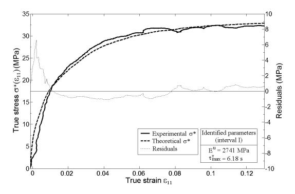
Figure 6: Experimental data, fitted curve (equation 15) and residuals obtained when identifying parameters  $E^u$  and  $\tau_{\max}^T$  on interval I (Specimen  $A_{//}$  - Strain rate of  $5 \times 10^{-3} \, \text{s}^{-1}$ ).
