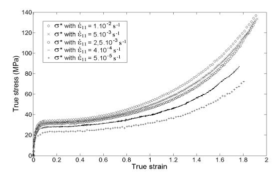
Figure 3: True stress  $\sigma^*$  versus true strain  $\mathcal{E}_{11}$  curves for different strain rates (Specimen  $A_{/\!/}$  ).
