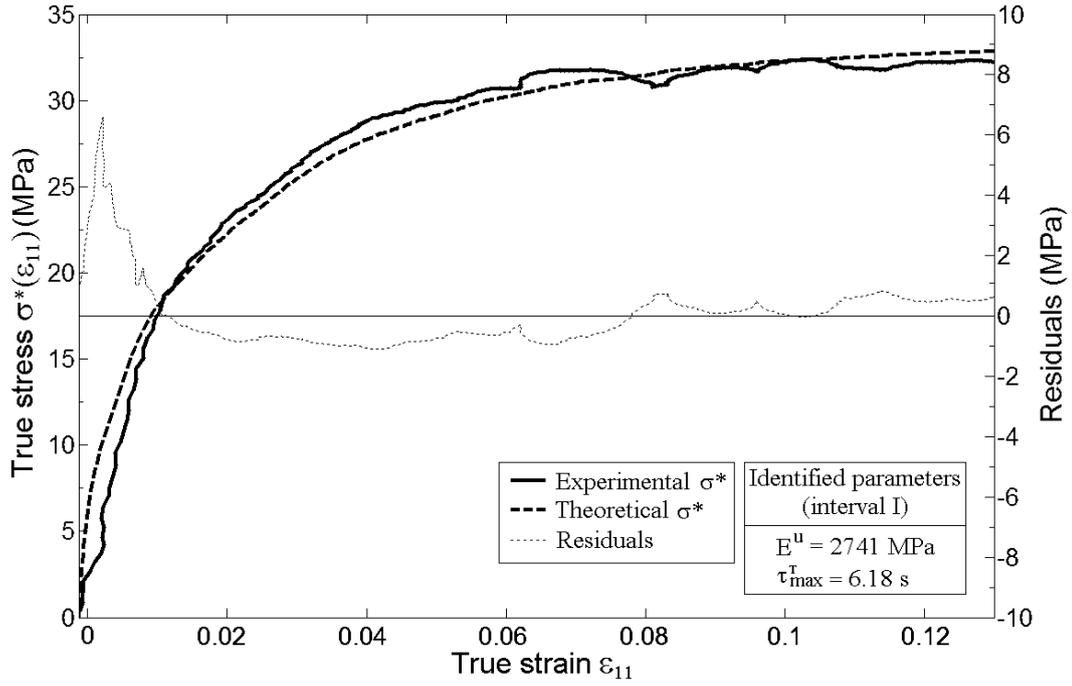
Figure 6: Experimental data, fitted curve (equation 15) and residuals obtained when identifying parameters  $E^u$  and  $\tau_{\max}^T$  on interval I (Specimen  $A_{//}$  - Strain rate of  $5 \times 10^{-3} s^{-1}$ ).
