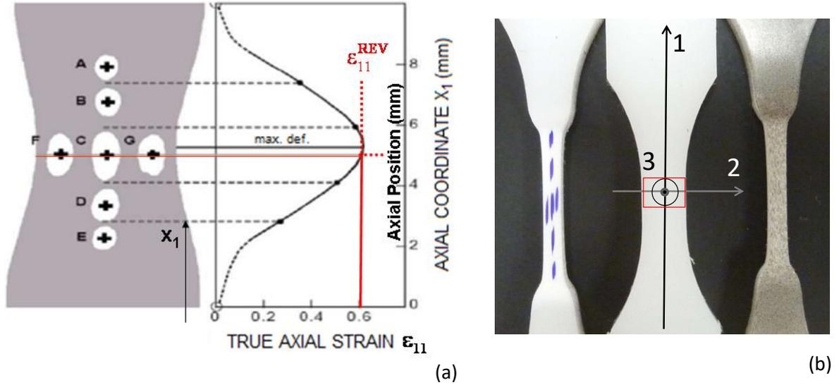
Figure 1: a) Principle of the true strain measurements as put into action in the VidéoTraction system. b) Pictures of the specimen in non-deformed (left) and highly-deformed (right) states.
