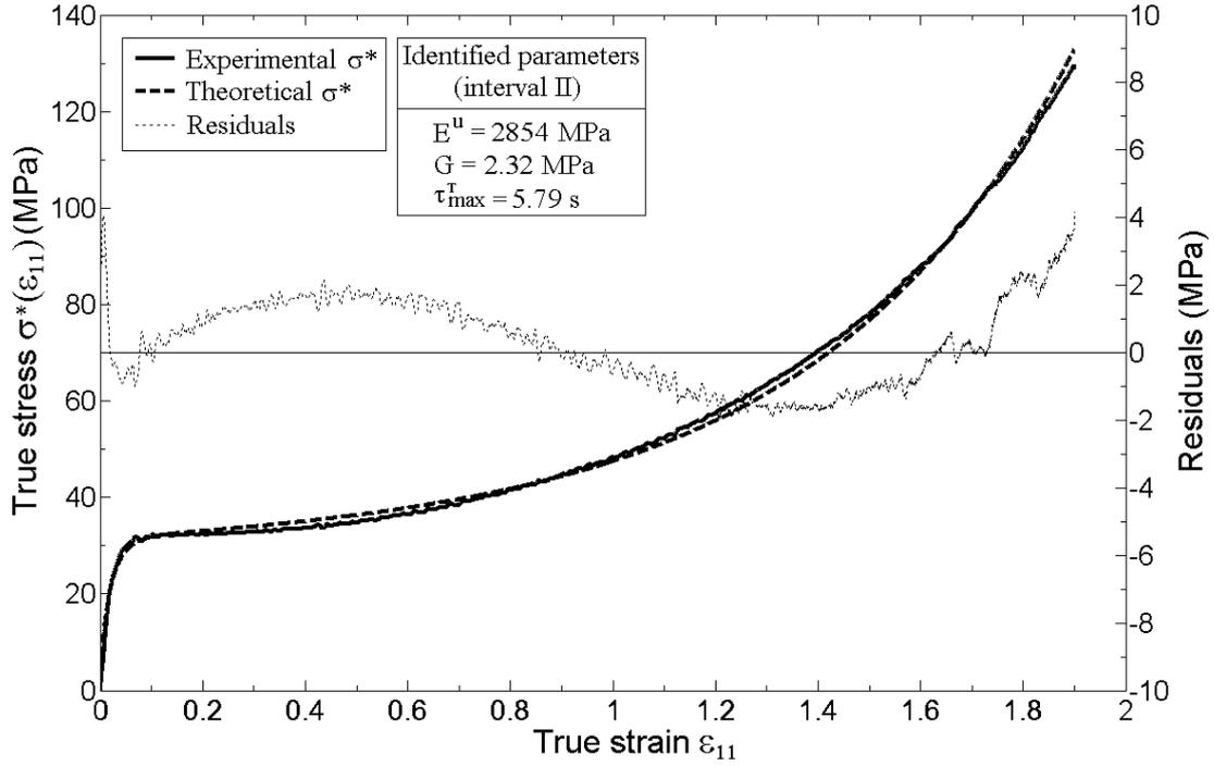
Figure 8: Experimental data, fitted curve (Eq. 15) and residuals obtained when identifying parameters  $E^u$ ,  $G$  and  $\tau_{\max}^T$  on interval II (Specimen  $A_{//}$  - Strain rate of  $5 \times 10^{-3} s^{-1}$ ).
