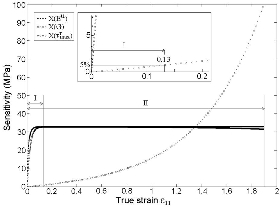
Figure 10: Normalized sensitivities to  $E^u$ ,  $G$  and  $\tau_{\max}^T$  parameters on interval II.
