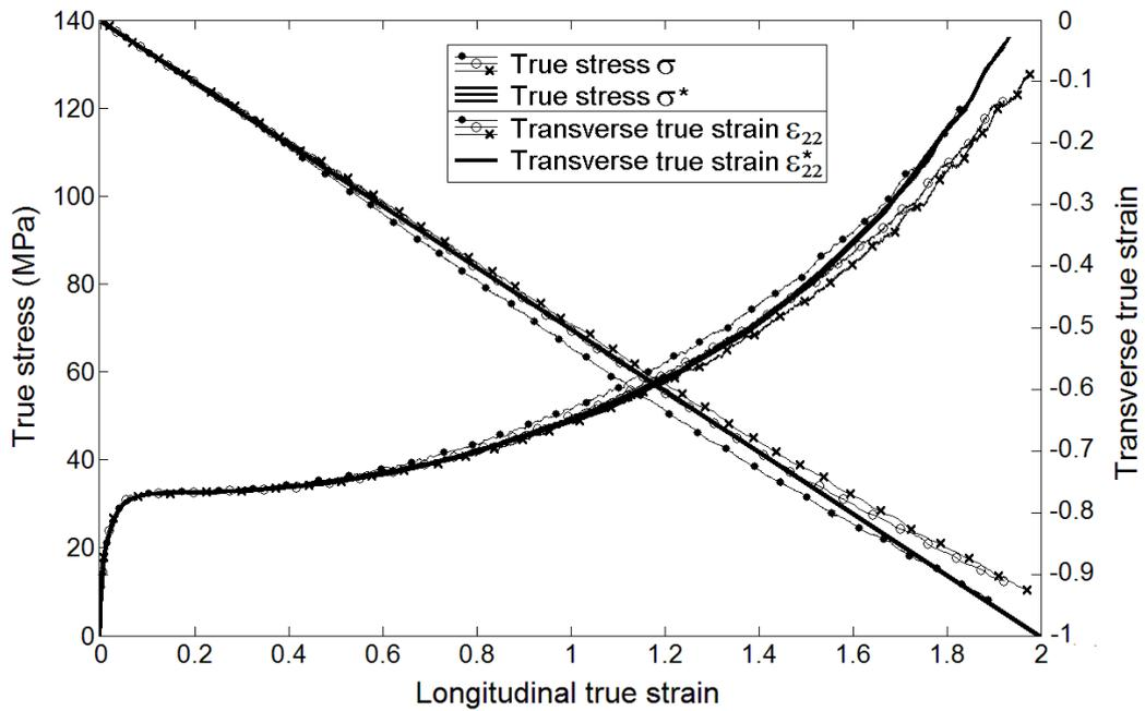
Figure 2: True stress  $\sigma$  or  $\sigma^*$  (left axis - the latter in solid black) and transversal true strain  $\varepsilon_{22}$  (right axis), plotted versus longitudinal true strain  $\varepsilon_{11}$  for 3 repeated experiments – Specimen  $A_{//}$  at  $\dot{\varepsilon}_{11} = 0.005 \text{ s}^{-1}$ .
