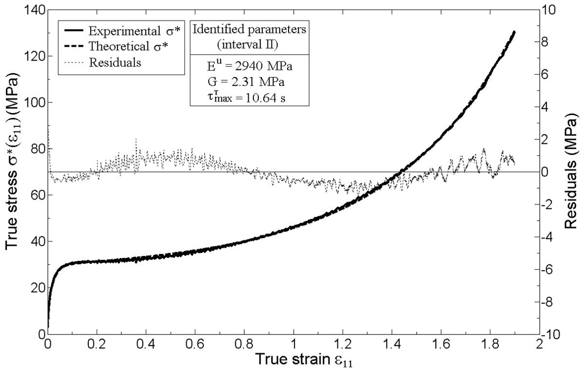
Figure 7: Experimental data, fitted curve (Eq. 15) and residuals obtained when identifying parameters  $E^u$ ,  $G$  and  $\tau_{\max}^T$  on interval II (Specimen  $A_{//}$  - Strain rate of  $2.5 \times 10^{-3} s^{-1}$ ).
