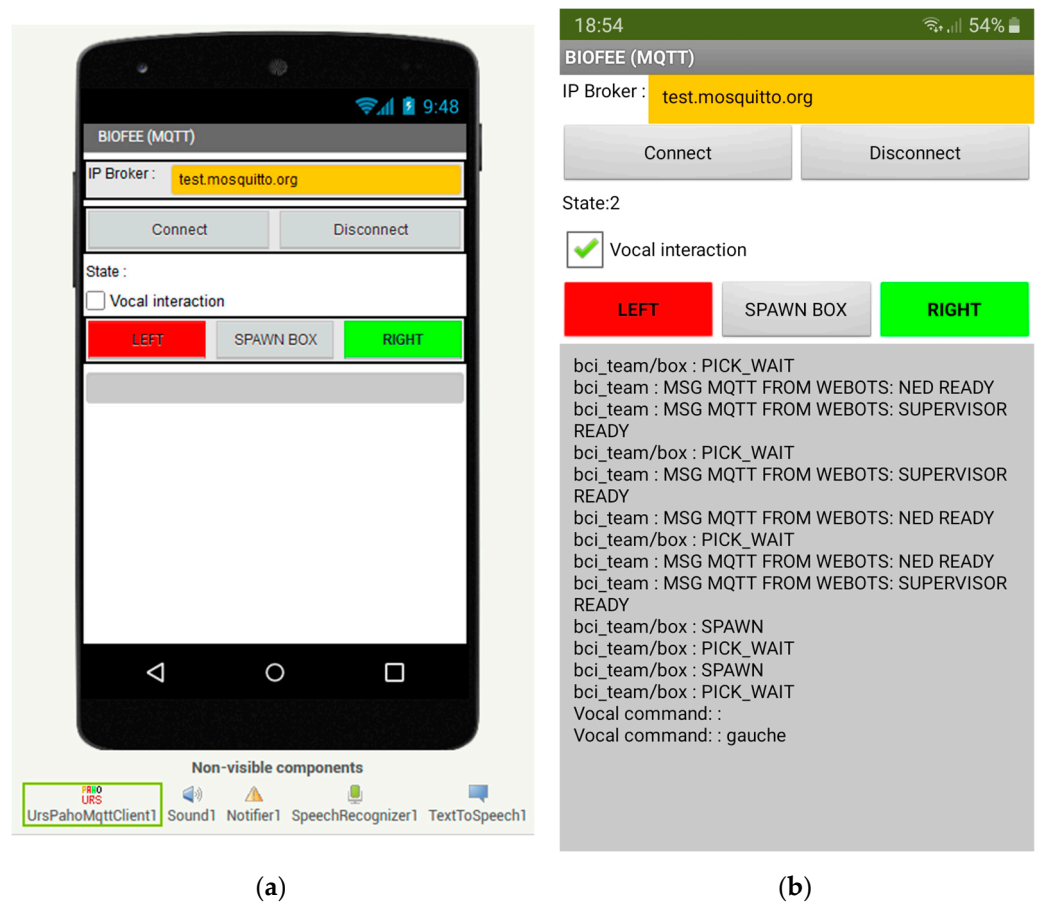
Figure 14. App Inventor mobile application connected to MQTT to interact with the Webots Ned cobot. (a) Designer view; (b) Android APK executable version.
