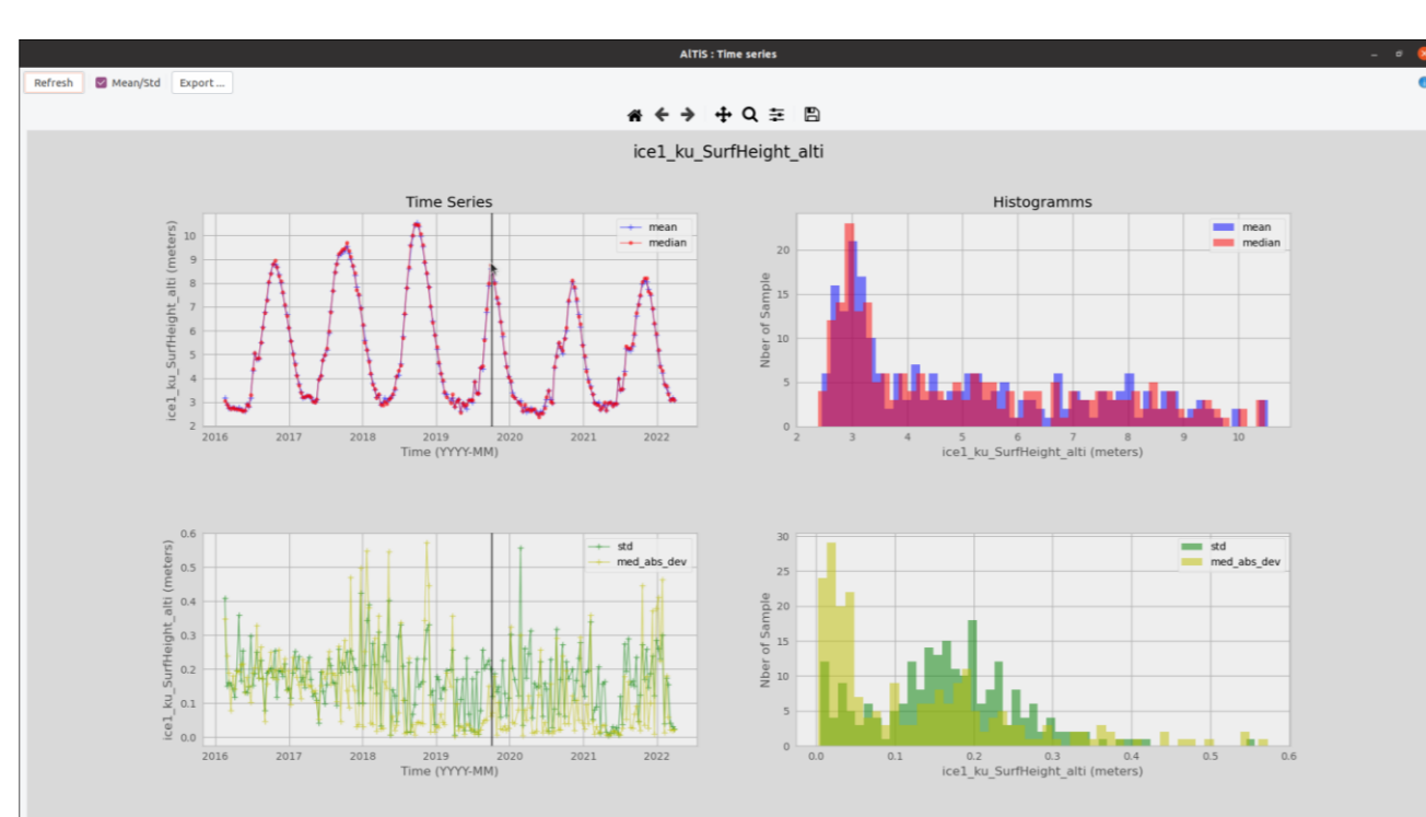
Screenshot of AITiS GUI : 4 displays windows in order to edit altimeter measurement graphically
