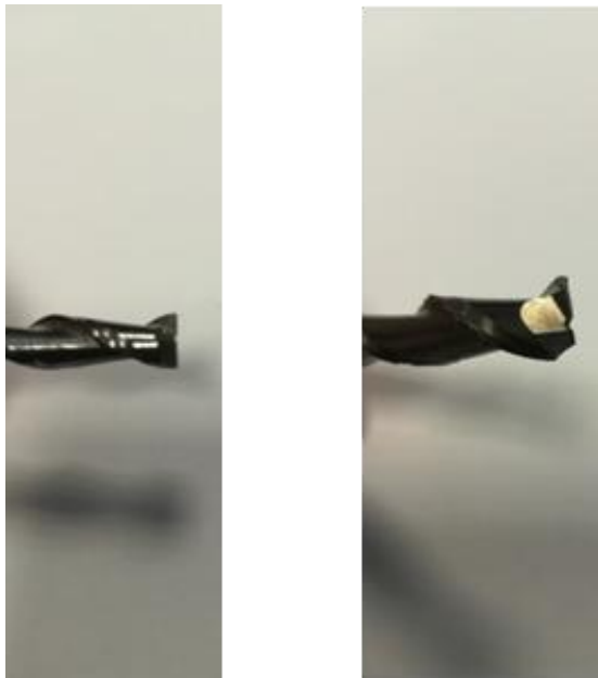
Fig. 2. Good milling tool (left) and damaged milling tool (right)
