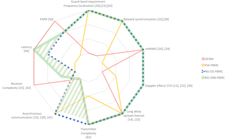
FIGURE 8: Radar chart illustrating the set of 6G-IoT relevant KPI and tradeoffs for OFDM and several variants of the original and NG-FBMC waveforms. A larger circle radius represents a better system performance. The green shaded area corresponds to the flexibility that can be attained by the NG-FBMC receivers, according to the selected parameters N_s and N_{UF} .
