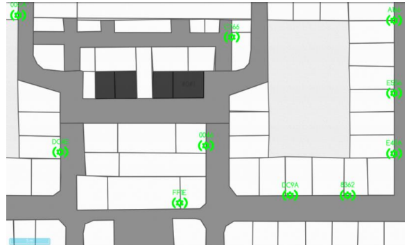
Fig. 10. Localization of the radio modules in the emergency department.
