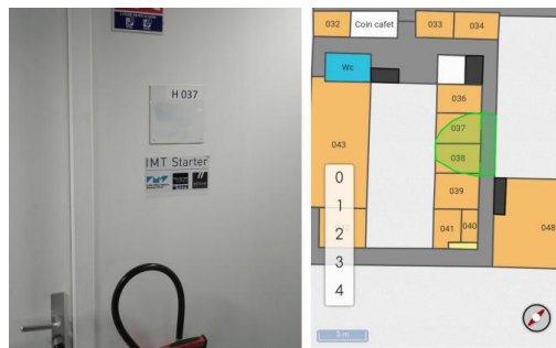
Fig. 3. The coupling principle between the cartography and the localization: the green surface is the resulting localization and requires no calibration or model design. On the left hand side the picture of what the smartphone "sees" and on the right hand side the restitution of the proposed system
