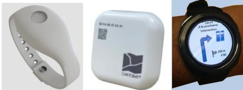
Fig. 4. A possible wearable for hospitals: a wristband (left), a simple tag for the stratcher (middle), and a guiding watch (right).
