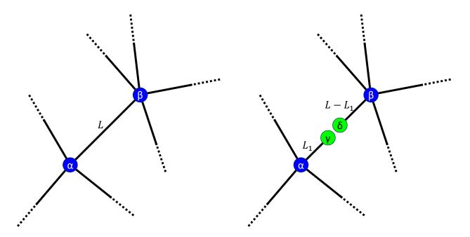
FIG. 1. Considered fault: the cable linking nodes  $\alpha$  and  $\beta$  is interrupted (cut) at a distance  $L_1$  from  $\alpha$ , creating two new nodes  $\gamma$  and  $\delta$ . The sketches on the left and right show, respectively, the intact and faulty cable of interest within a larger transmission-line network.
