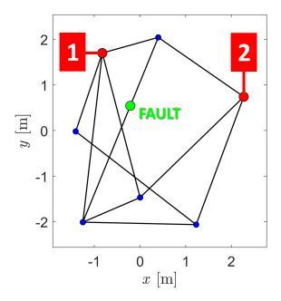
FIG. 3. The considered random transmission-line network. Each of the two red nodes is directly connected to one asymptotic scattering channel. The location of the fault, at which the faulty cable is interrupted, is highlighted in green.
