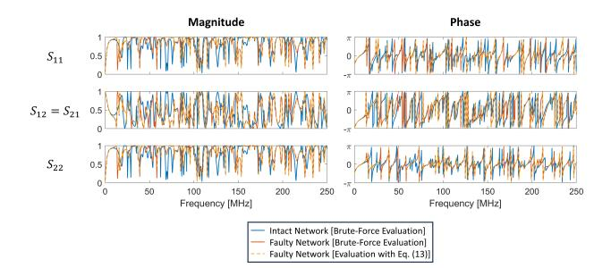
FIG. 4. Comparison of the frequency-dependent scattering coefficients in terms of magnitude (right) and phase (left) for the intact network (blue), the faulty network (red), and the faulty network evaluated with Eq. (13) (yellow).
