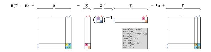
FIG. 2. Fault-induced update of the interaction matrix in the reduced  $n \times n$  basis. The update concerns the  $2 \times 2$  block of the interaction matrix involving nodes  $\alpha$  and  $\beta$ .
