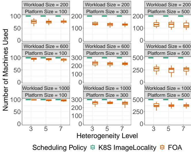
Figure 7: Comparison of K8S ImageLocality and FOA in terms of the number of machines used (y-axis) against the heterogeneity level (x-axis).
