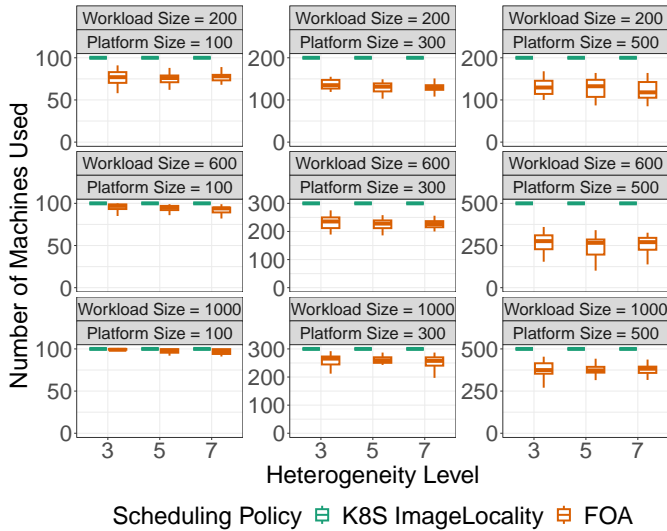
Figure 7: Comparison of K8S ImageLocality and FOA in terms of the number of machines used (y-axis) against the heterogeneity level (x-axis).
