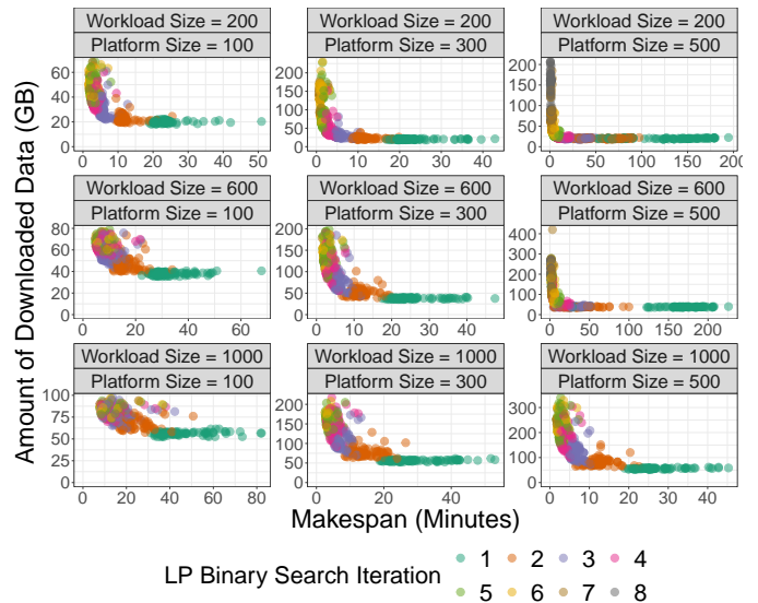
Figure 4: FOA 's linear program trade-off between makespan (x-axis) and amount of downloaded data (y-axis). The color of the points represents the iteration-id of the linear program binary search. Each one is one solution of the linear program.
