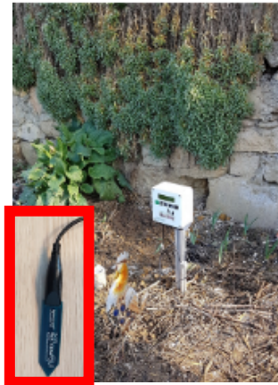
Installation of soil moisture sensors
