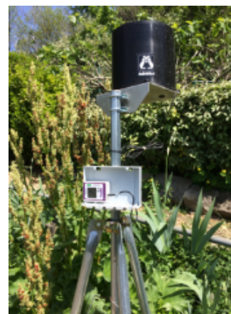
Automatic tipping bucket rain gauge.
