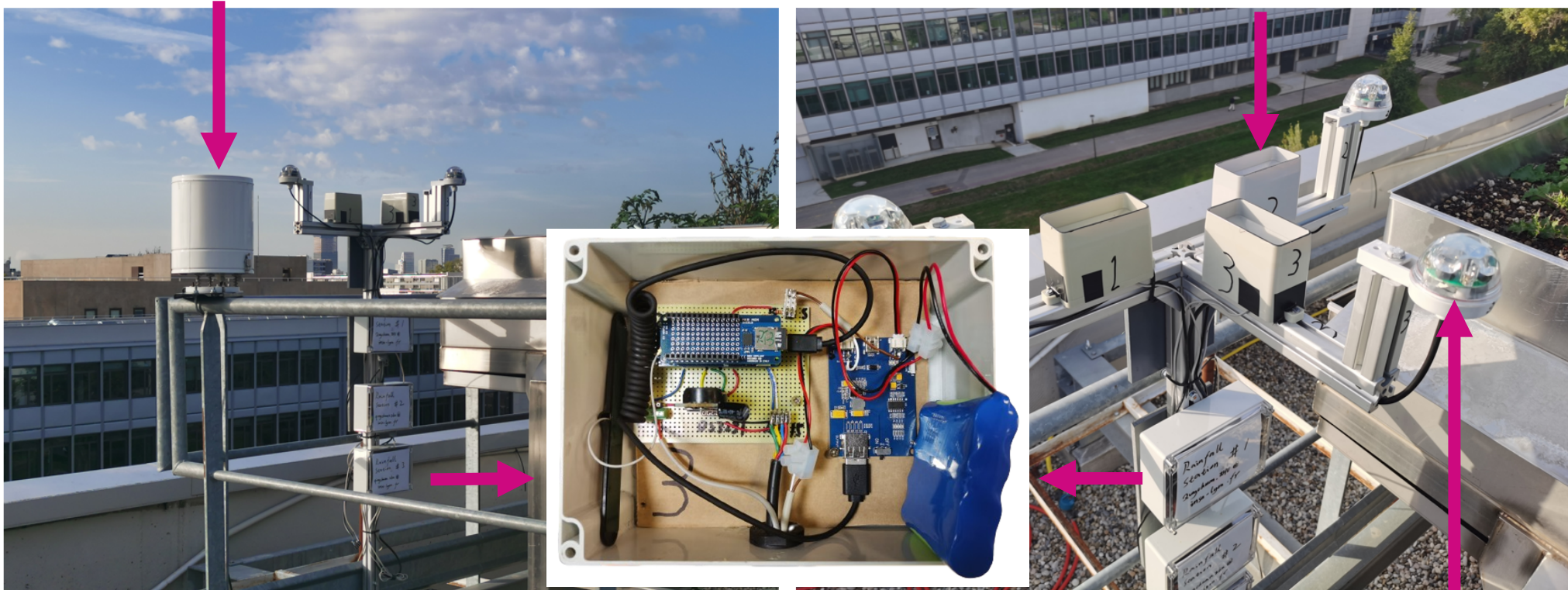
Waterproof box contains hardware Optical rain gauge RG-15
