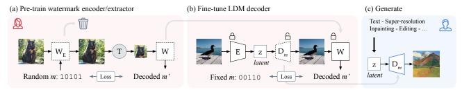
Figure 2. Steps of the method. (a) We pre-train a watermark encoder  $W_E$  and extractor W, to extract binary messages. (b) We fine-tune the decoder  $\mathcal{D}$  of the LDM's auto-encoder with a fixed signature m such that all the generated images (c) lead to m through W.
