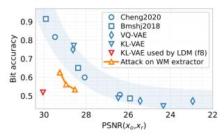
Figure 7. **Removal attacks.**  $x_o$  is the image produced by the original generator,  $x_r$  is the version produced by the watermarked generator and then attacked. Bit accuracy is on the watermark extracted from  $x_r$ . Neural auto-encoders [4, 11, 20] follow the same trend, except with the one used by LDM ('KL-f8' for our LDM). When access to the watermark extractor is granted, adversarial attacks also remove the watermark at lower PSNR budget.
