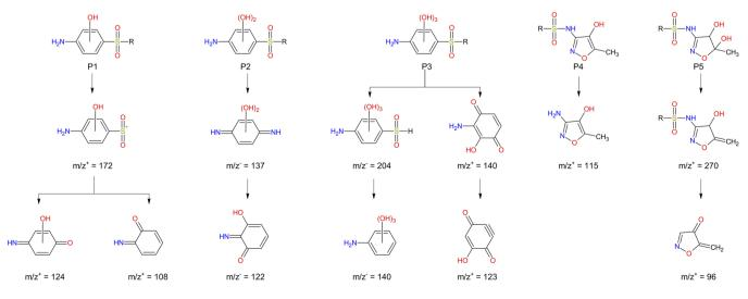
**FIGURE 4** MS/MS fragmentation patterns of the hydroxylated degradation products of sulfamethoxazole obtained during plasma treatment.
