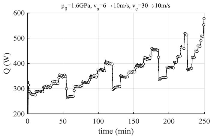
Figure 10: Friction losses during the first test
