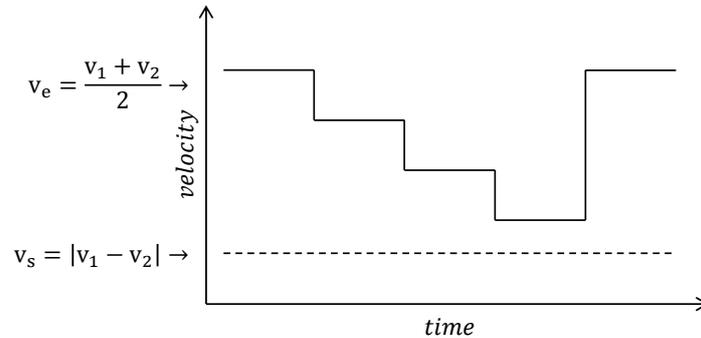
Figure 5: Surface speed parameters during the test block
