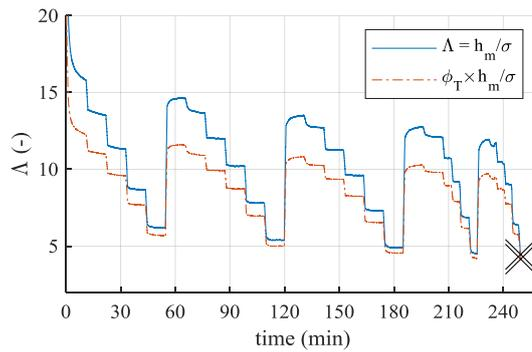
Figure 17: Reduced film thickness evolution during the test
