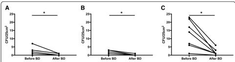
**Fig. 3** The importance of an adequate biodecontamination on microbiological qualification. Microbiological qualification results on 3 areas of interest: the carousel with ISO4.8 specifications (**a**), the reservoir surface (**b**) and the gloves (**c**) both with ISO7 specifications, before and after biodecontamination (BD). \*P < 0.05, n = 7; two-tailed Wilcoxon matched-pairs signed rank test.
