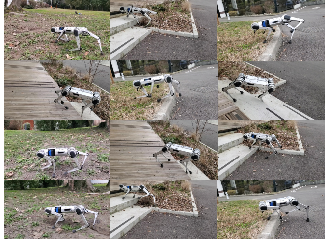
Fig. 1: Snapshots of the proposed low-level policy controlling the Mini-Cheetah through different challenging terrains. Full video can be found at: https://youtu.be/B92HB964xq8
