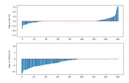
**Figure 4.** Solution quality variation on jobshop instances. The gap is computed as  $\frac{(m_1-m_2)\times 100}{min(m_1,m_2)}$  where  $m_1$  is the makespan of the solution found by ARIES and  $m_2$  is the makespan of the solution found by CPOPTIMIZER (resp. MISTRAL). A negative value indicates that ARIES returned a strictly better solution.
