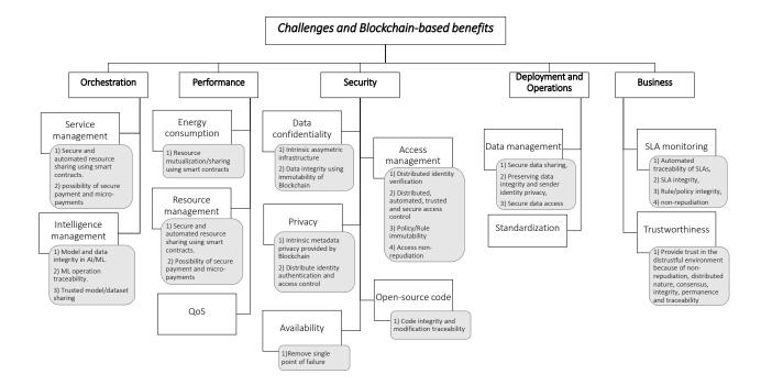
Fig. 3. O-RAN challenges and the possible benefits of Blockchain technology to address them. The gray boxes indicate Blockchain-based solutions for respective challenges. Note that, to the best of our knowledge, there is a lack of sufficient resources regarding the usage of Blockchain in QoS and Standardization areas.
