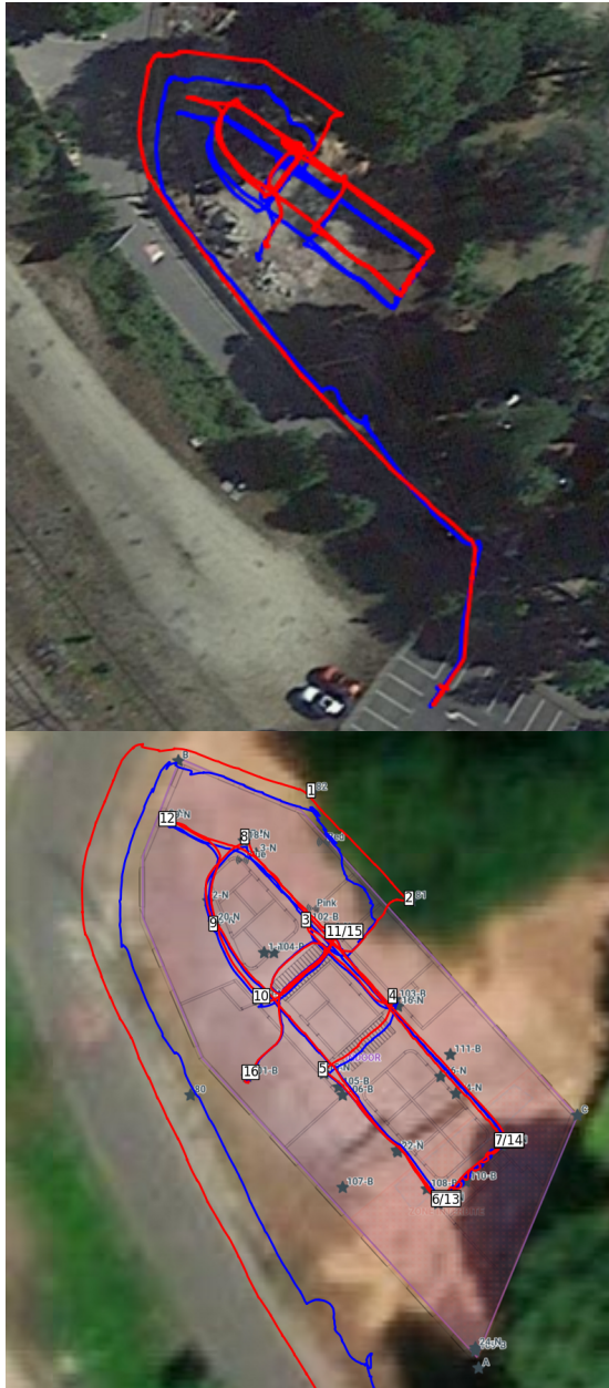
Fig. 3: Outdoor + Indoor trajectory using classic magnetoinertial (blue) and step-detection aided (red) navigation. Above: full trajectory, below: zoom on building plan (with cancelled outdoor drift).
