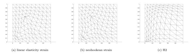
Figure 12: three-point registration; visualization of the deformed meshes for three choices of the objective function in (10).
