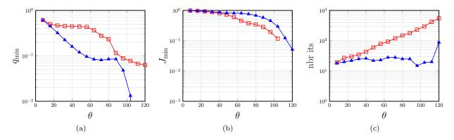
Figure 8: Large deformation mesh morphing. Behavior of the minimum radius ratio  $q_{\min}$ , the minimum Jacobian  $J_{\min}$ , and the number of iterations for exp-jac and exp-mesh objective function and for several values of  $\theta$ . ( $\delta = 10^{-6}$ ,  $\epsilon = 0.05$ ,  $\kappa_{\text{msh}} = 10$ ,  $n_{\text{lp}} = 25$ ). exp-mesh  $\Box$ ; exp-jac  $\triangle$ .
