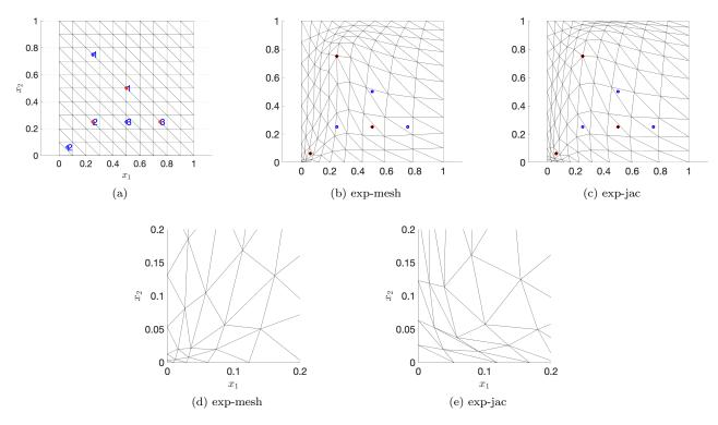
Figure 3: three-point registration problem; visualization of the reference mesh and of the deformed mesh for two different registration algorithms ( $\delta = 10^{-6}$ ,  $\epsilon = 0.1$ ,  $\kappa_{\rm msh} = 10$ ). Figures (d)-(e) show a zoom of the deformed meshes in the proximity of the origin.
