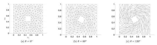
Figure 7: large deformation mesh morphing. (a) reference configuration. (b)-(c) deformed meshes obtained using (10) with exp-mesh objective,  $\delta = 10^{-6}$ ,  $\kappa_{\rm msh} = 10$ ,  $n_{\rm lp} = 25$ .
