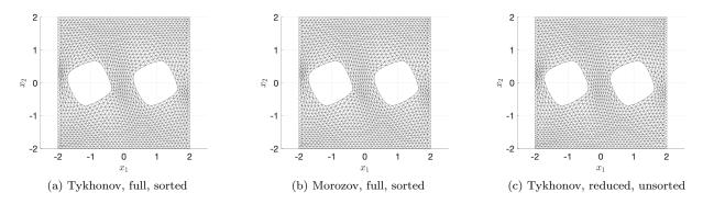
Figure 11: geometry reduction of a parametric two-dimensional domain. Deformed mesh obtained using three different methods for  $\mu = [\nu_{\text{max}}, \nu_{\text{max}}]$ .
