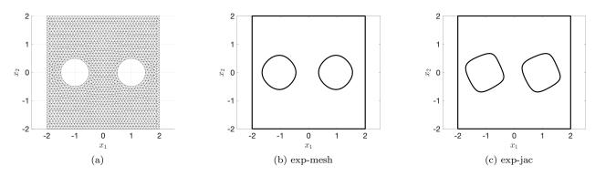
Figure 9: geometry reduction of a parametric two-dimensional domain. (a) reference configuration. (b) domain  $\Omega_{\mu}$  for  $\mu = [\nu_{\min}, \nu_{\min}]$ , with  $(\nu_{\min})_j = \min_{\nu \in \mathcal{P}_{\text{in}}}(\nu)_j$ , j = 1, 2, 3. (c) domain  $\Omega_{\mu}$  for  $\mu = [\nu_{\max}^{(1)}, \nu_{\max}^{(2)}]$ , with  $(\nu_{\max})_j = \max_{\nu \in \mathcal{P}_{\text{in}}}(\nu)_j$ , j = 1, 2, 3.
