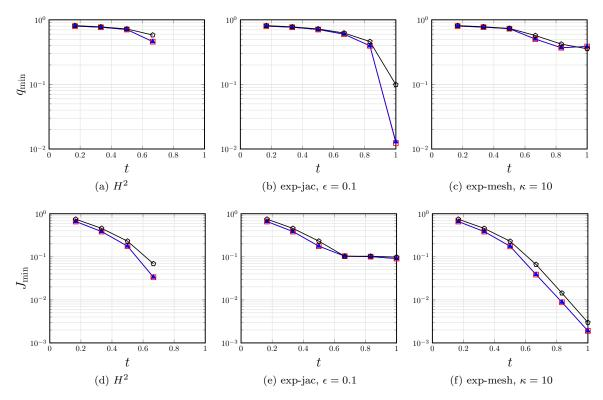
Figure 4: three-point registration problem. Performance of the Morozov-regularized statement (10) for the objective functions H2, exp-jac and exp-mesh, for three choices of  $\delta$  and for the deformation points  $\{y_i(t) = (1-t)x_i + ty_i\}_{i=1}^3$  for  $t \in [0,1]$ .  $\delta = 10^{-6}$  ;  $\delta = 10^{-4}$ ,  $\delta = 10^{-2}$  .
