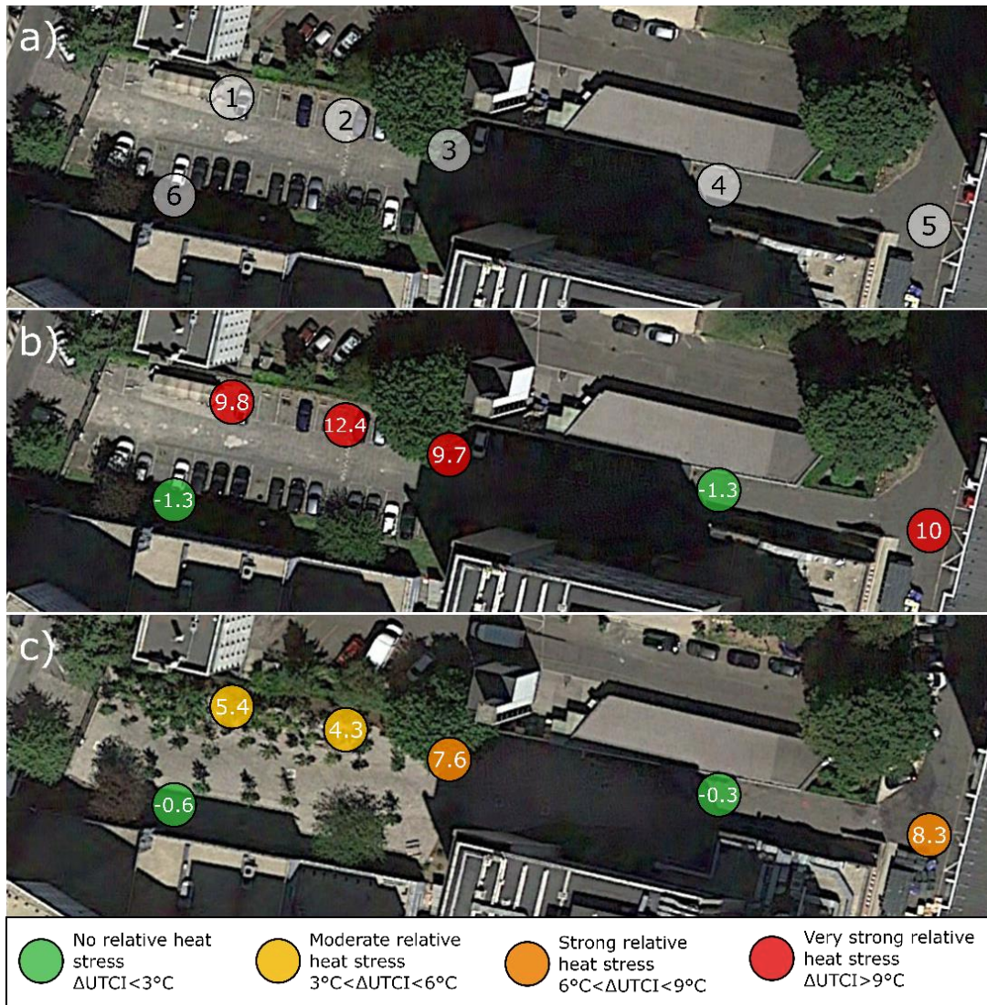
Figure 13: a) Measurement points, b) thermal over-stress before renovation (June 2018), c) thermal over-stress after renovation (September 2021).
