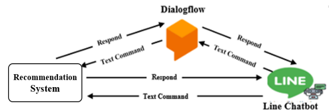
Fig. 2. LINE chatbot with DialogFlow and recommendation system architecture
