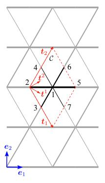
Figure 2: 2D architectured material (grey lines) and unit cell  $\mathcal{C}$  (dashed red lines).
