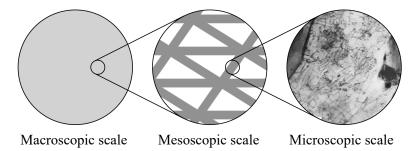
Figure 1: The three different scales of description of a architectured material.
