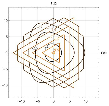
Figure 11: Isovalues of the limit surface of the linear elasticity domain in the deviatoric deformation space (x1000). Isovalues are taken each 0.0015 along the spheric axis.
