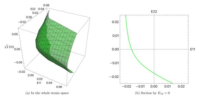
Figure 8: Limit surface associated with the aperiodic buckling.
