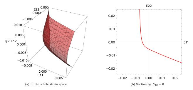
Figure 5: Limit surface associated with the periodic buckling.
