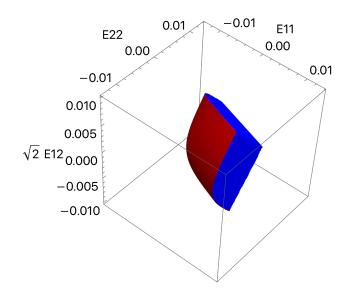
Figure 10: Domain of linear elasticity for the equilateral triangle lattice limited by the material non linearity limit surface  $(\blacksquare)$  and the periodic buckling limit surface  $(\blacksquare)$  in the canonic basis.
