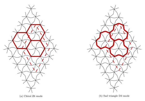
Figure 6: Buckling modes of the regular triangular cell architectured material under equi-biaxial compression. In dashed red line: contour of the 3x3 periodic pattern. In solid red line: contour of specific mode shape identified by [22].
