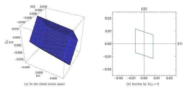
Figure 4: Limit surface associated with the limit of elasticity of the constitutive material.
