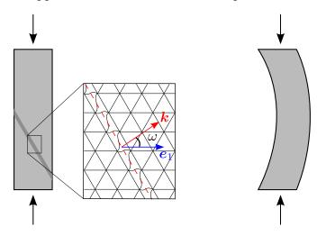
Figure 7: Aperiodic instabilities: (left) shear band along a band of normal k, (right) global buckling of the structure.
