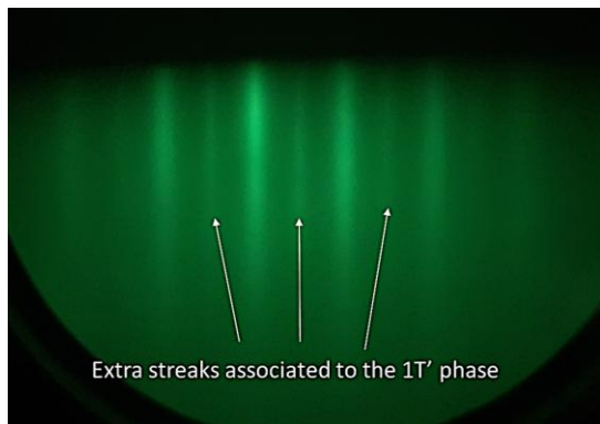
Figure 1: RHEED pattern observed on 3 MLs WSe 2 deposited on GaP(111)B at 250°C.
