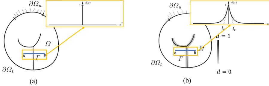
Figure 1: A solid body  $\Omega$  with the crack set  $\Gamma$ : (a) conventional sharp cracks and (b) diffuse crack bands in phase-field.
