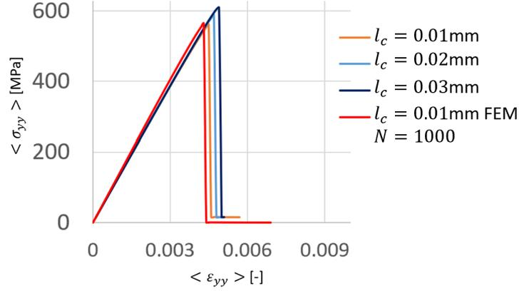
Figure 8: Results of Wu’s phase-field model for single notch model with different  $l_c$  values. ( $G_c^e/G_c = 1.$ )
