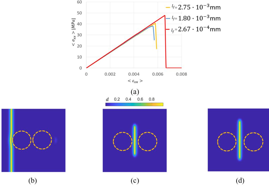
Figure 14: Results of Wu's phase-field model for two-fibers unit-cell composite model ( $l_c = 5.00 \cdot 10^{-4}$ mm): (a) Averaged stress-strain curves; (b) Local crack patterns for  $l_f = 2.67 \cdot 10^{-4}$ mm; (c) Local crack patterns for  $l_f = 1.80 \cdot 10^{-3}$ mm; (d) Local crack patterns for  $l_f = 2.75 \cdot 10^{-3}$ mm. (Remark: The orange dash circles are fiber contours.)
