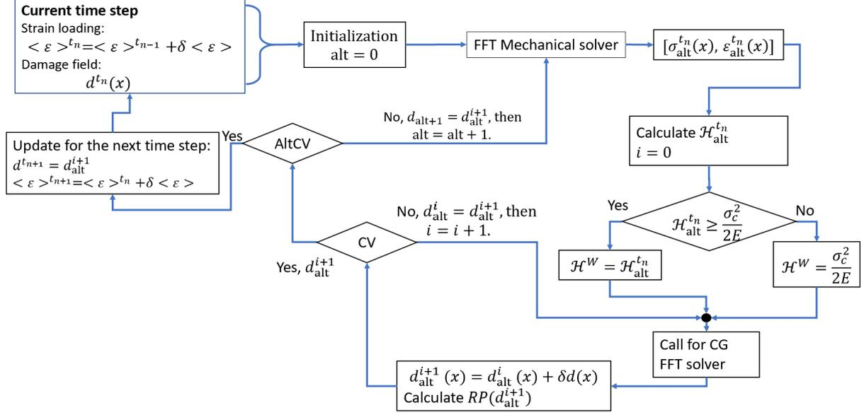
Figure 4: The flow chart of Wu's phase-field method based on the Newton-Krylov algorithm in FFT solver. (remark: CV is damage field convergence check. AltCV is alternating minimization convergence check.)
