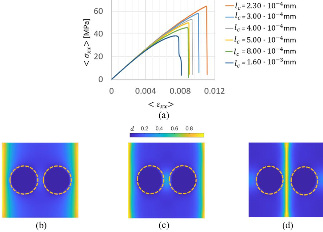
Figure 11: Results of Miehe's phase-field model for two-fibers unit-cell composite model ( $l_f = 2.75 \cdot 10^{-3}$ mm): (a) Averaged stress-strain curves; (b) Local crack patterns for  $l_c = 1.60 \cdot 10^{-3}$ mm; (c) Local crack patterns for  $l_c = 8.00 \cdot 10^{-4}$ mm; (d) Local crack patterns for  $l_c = 5.00 \cdot 10^{-4}$ mm. (Remark: The orange dash circles are fiber contours.)
