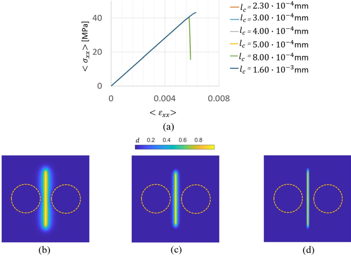
Figure 12: Results of Wu's phase-field model for two-fibers unit-cell composite model: (a) Averaged stress-strain curves ( $l_f = 2.75 \cdot 10^{-3}$ mm); (b) Local crack patterns for  $l_c = 8.00 \cdot 10^{-4}$ mm; (c) Local crack patterns for  $l_c = 5.00 \cdot 10^{-4}$ mm; (d) Local crack patterns for  $l_c = 2.30 \cdot 10^{-4}$ mm. (remark: the curves for  $8.00 \cdot 10^{-4}$ mm to  $2.30 \cdot 10^{-4}$ mm are superimposed. The orange dash circles are fiber contours.)
