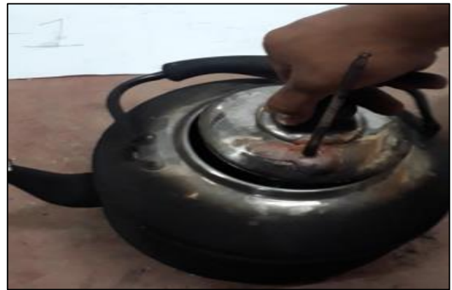
Figure-3. Kettle installed with thermometer.
