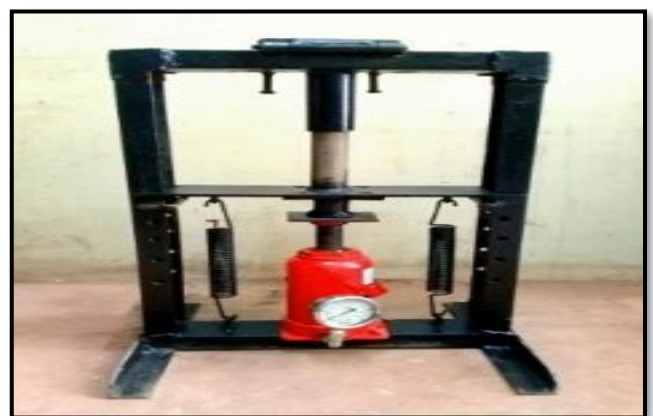
Figure-1. Single mold manual hydraulic briquetting device.
