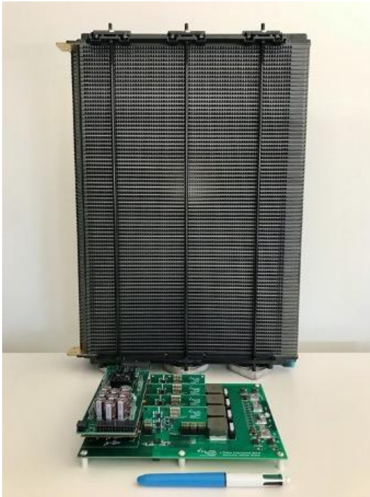
Fig. 1 IBC4 prototype in front of an air-cooled 80-cell/ 3.3 kW open-cathode PEM fuel cell.
